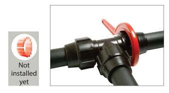
Open split ring and place on pipe with lugs touching bush. Reuse split rings only twice, blunt rings will not bite into pipe.
