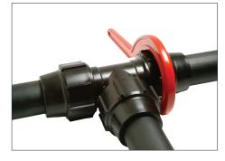
Do not use a wrench with handle lengths longer than standard Plasson C spanners. For 63mm: max. handle length should be 22cms. For 75–125mm: max. handle length should be 46cms.
