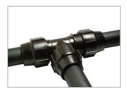
Open split ring and place on pipe with lugs touching bush. Reuse split rings only twice, blunt rings will not bite into pipe.
