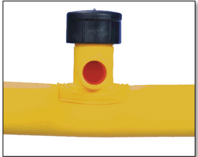
Excessive Heating and/or Overpressurization of joint
