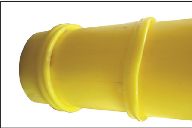
Pressure fluctuation, misalignment over pressurization
